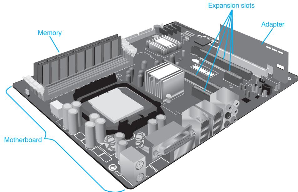
**FIGURE 1.21** Motherboard with expansion slots and an adapter
