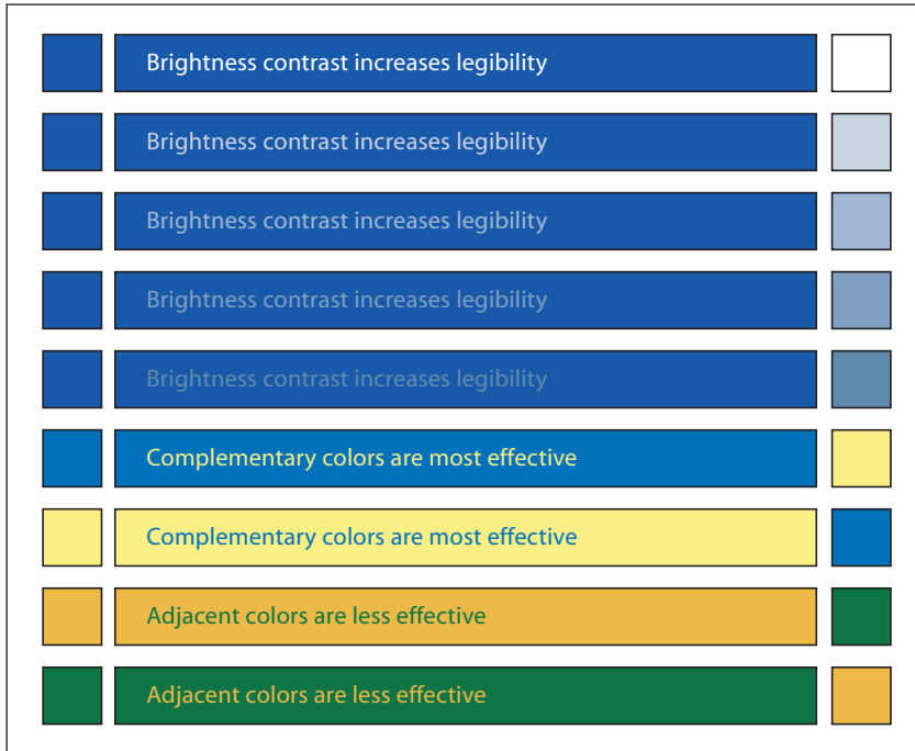
FIGURE 11.2 Text is most legible when foreground and background colors differ in brightness. As brightness contrast diminishes, so does legibility. Hue also affects color differentiation. Complementary colors produce more contrast than colors that are adjacent on the color wheel.
