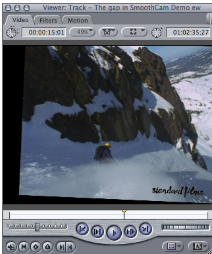
FIGURE 5: Note how much the picture has been rotated and shifted up and to the right to compensate for the excess camera movement.
