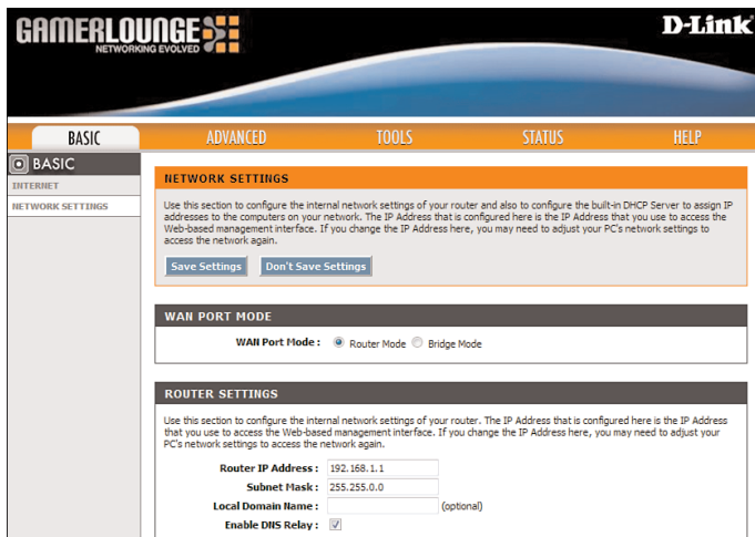
FIGURE 20.3 A typical router setup page.
