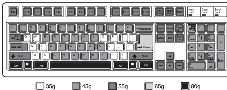
Figure 18.6 Force levels used on KeyTronicEMS keyboards with Ergo Technology.
