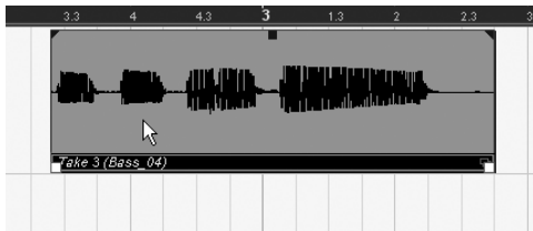
Figure 8.26 This event has been selected; the two triangles and small box at the top of the event will be moved to create a fade-in.
