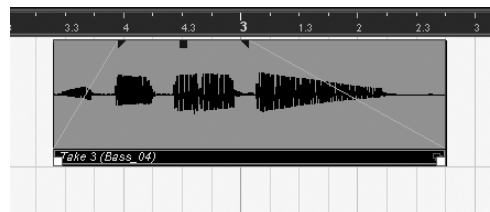
Figure 8.31 The fade-out is set; note that both the fade-in and fade-out are reflected in the change in the waveform.
