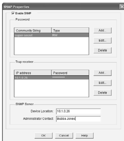
Figure 6-8 Using CCP to Configure SNMPv1 Information
