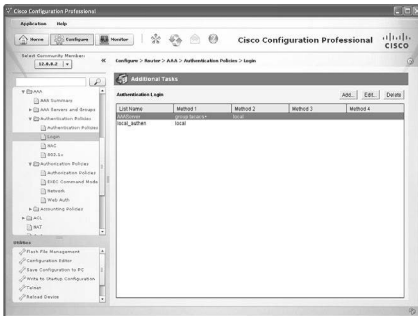
Figure 6-2 Using CCP to See Method Lists for Login
