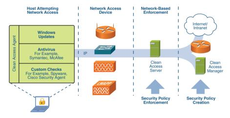
Unhealthy devices are placed in a "quarantine" wired or wireless network for remediation and are not permitted to access the rest of the production network. See Part V, "Securing the Network," for a more in-depth discussion of NAC and CCA.
