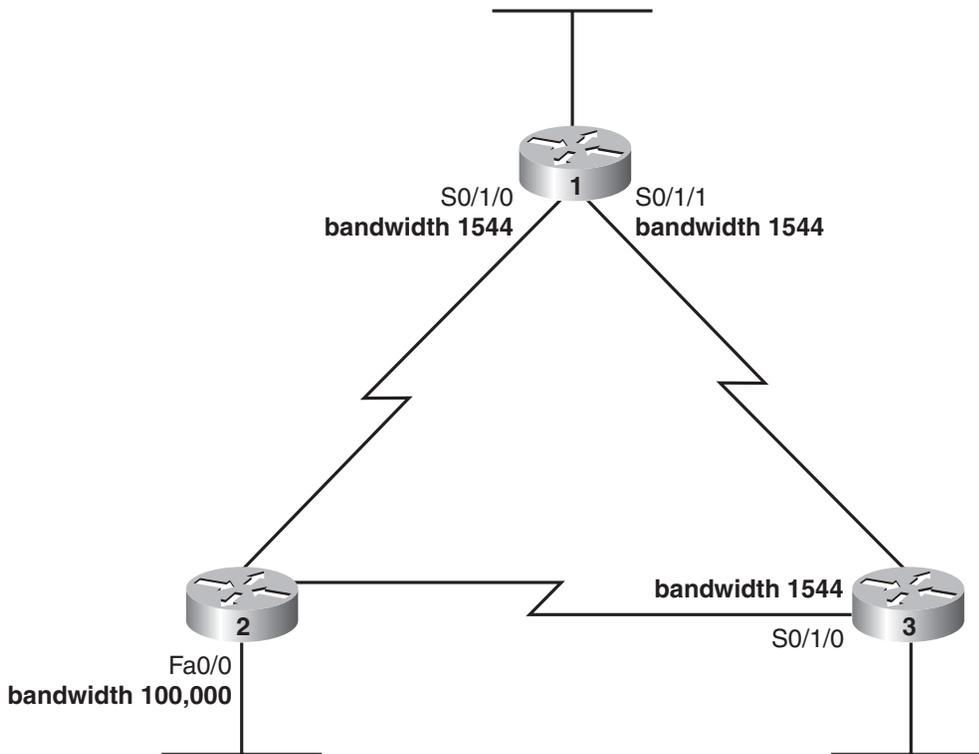
**Figure 6-4 Bandwidth and Delay Inputs into R1's Two Competing Routes for 172.22.12.192/26**
