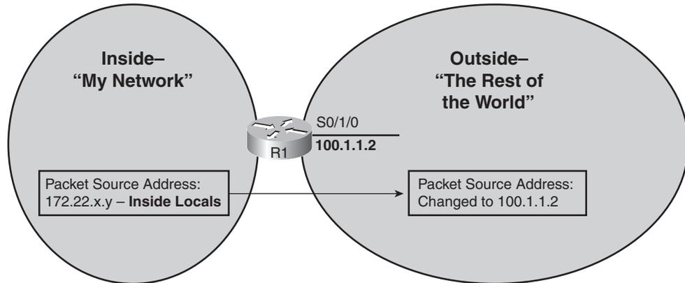
Figure 7-3 How NAT Overload Changes Inside Addresses and Ports
