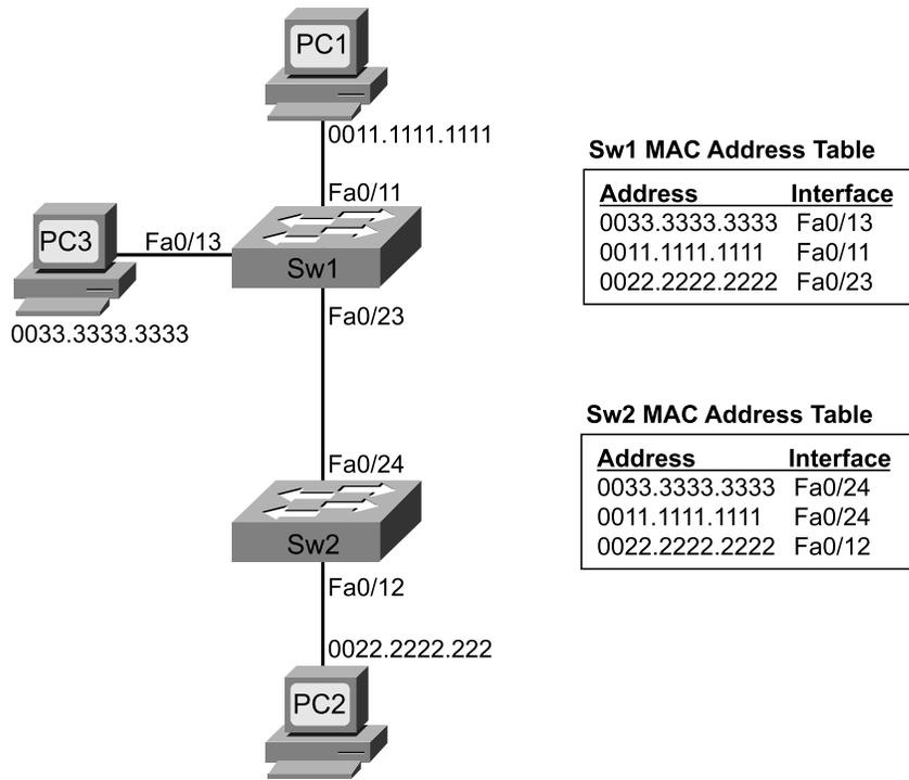
Figure 3-2 Forwarding Path and MAC Address Table Entries Used for Frames from PC3 to PC1
