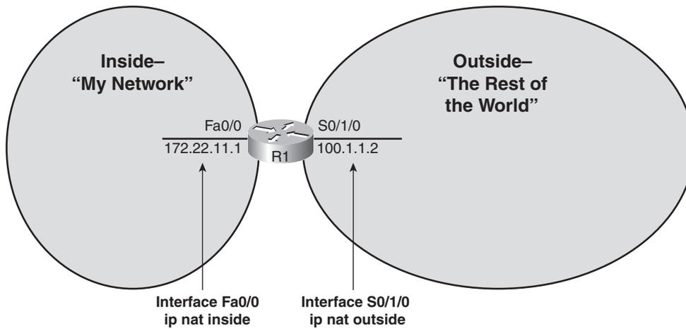
**Figure 7-6 Configuring NAT Overload Using an Interface as Inside Global**
