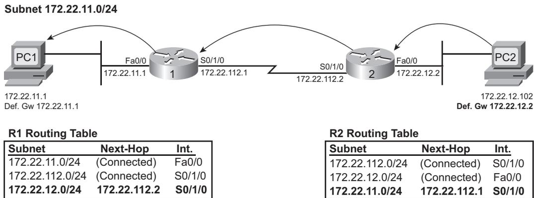
Figure 8-6 ip route Command with Outgoing Interface
