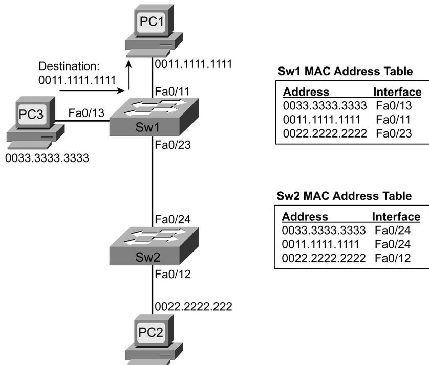
**Figure 3-3 Forwarding Path and MAC Address Table Entries Used for Frames from PC3 to PC2**
