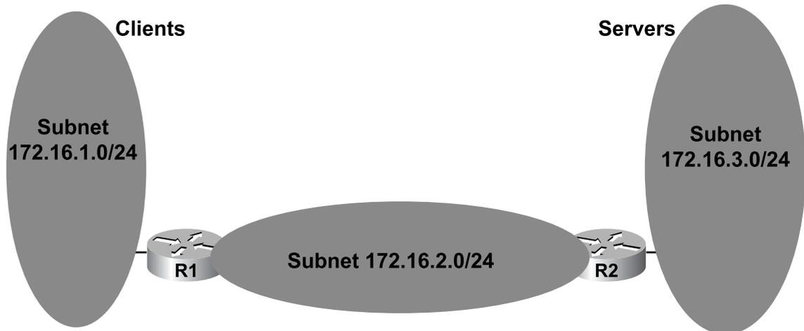
Figure 10-3 View of Packets That Should be Permitted by the ACL
