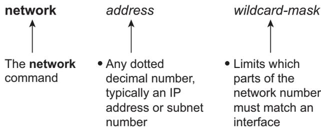
**Figure 5-5 The Impact of the EIGRP network Command – R1, Step 1**
