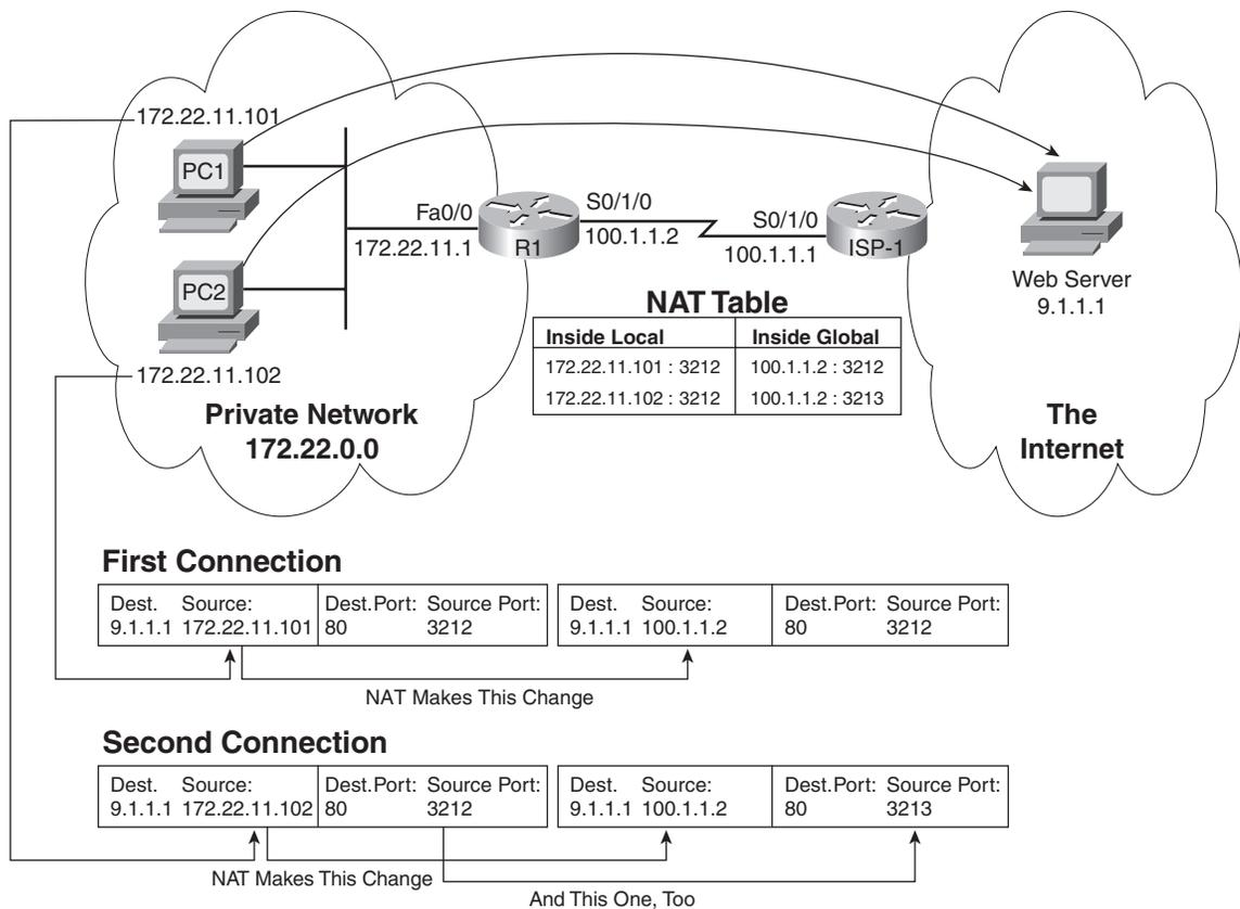
**Figure 7-4 Three TCP Connections Created to Test NAT Overload**
