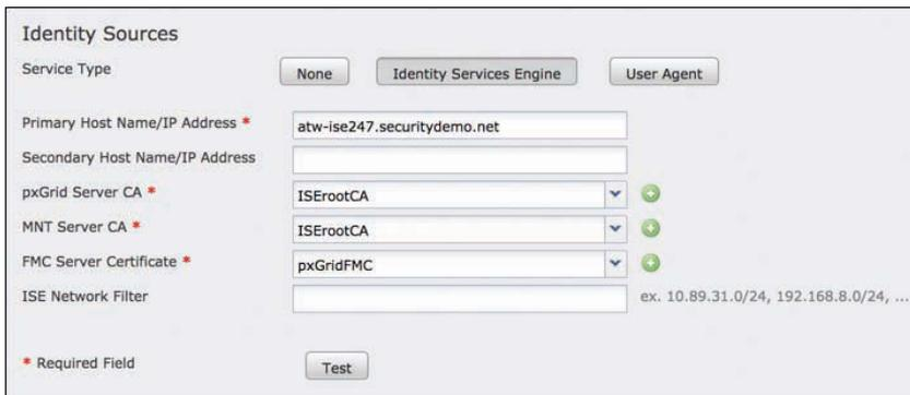
**Figure 6-19** Completed ISE Identity Source Form
