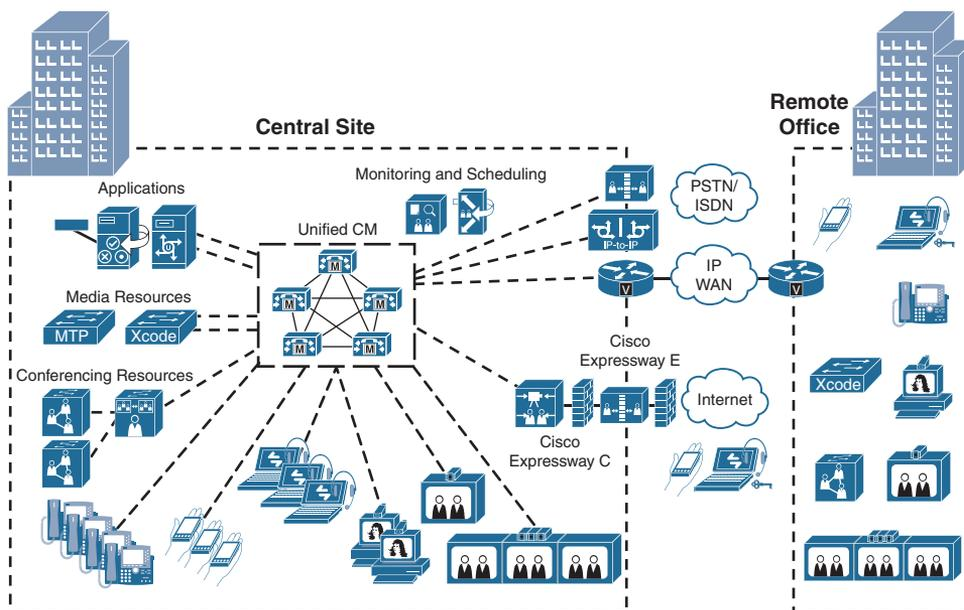
**Figure 2-2** Cisco Collaboration Solution Deployment at Campus and Branch in a Large Enterprise
