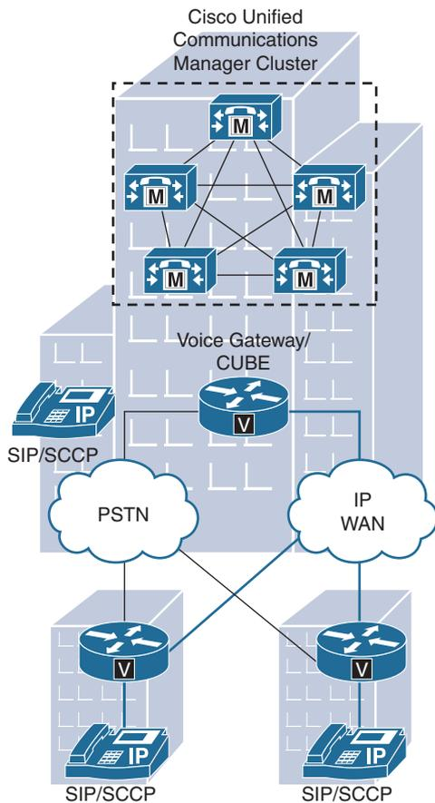
**Figure 2-4** *Centralized Multisite Deployment*
