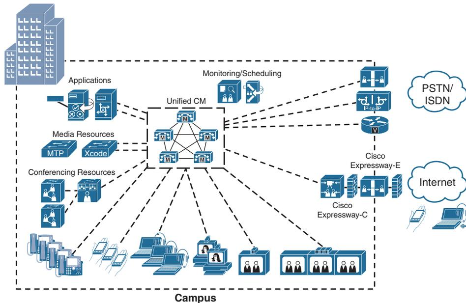
**Figure 2-1** *Cisco Collaboration Solution Campus Deployment in a Large Enterprise*
