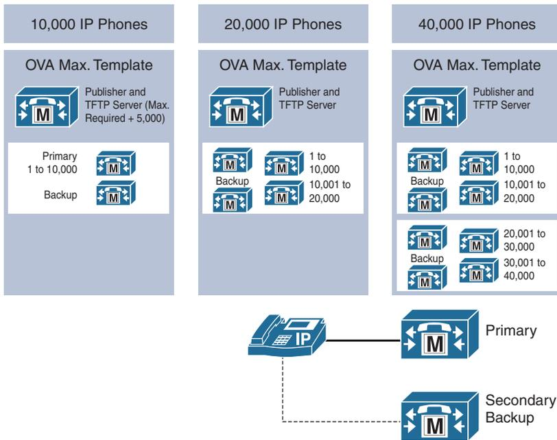
**Figure 2-11** 1:1 Redundancy Design
