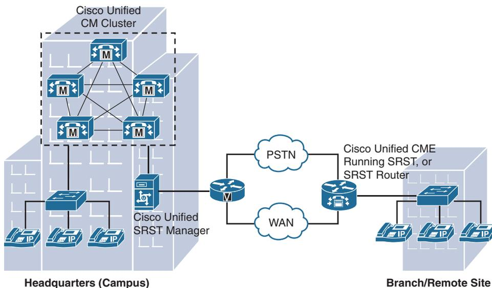
**Figure 2-5** Cisco Unified SRST/E-SRST Deployment with Centralized Call Processing
