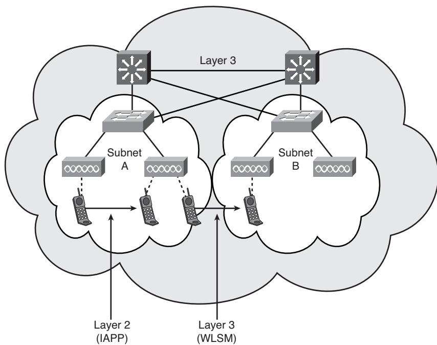
**Figure 11-14** Layer 2 Versus Layer 3 Roaming
