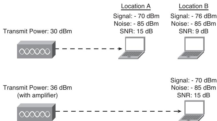
**Figure 11-5** Amplifiers Improve Range by Increasing Signal Strength
