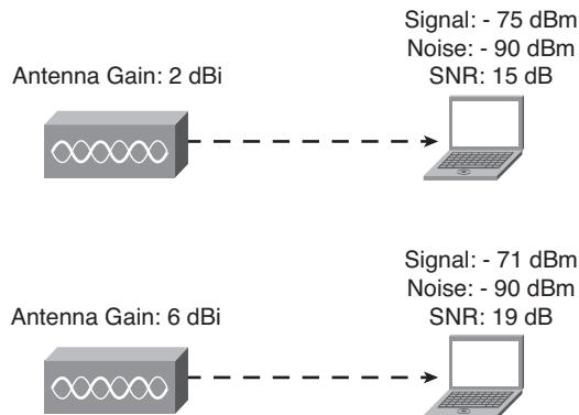
**Figure 11-10** Higher-Gain Antennas Boost Performance Throughout the Coverage Area
