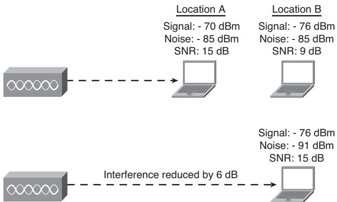
**Figure 11-7** Lowering Radio Signal Interference Increases Range
