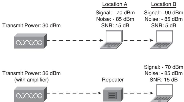
**Figure 11-6** Repeaters Extend Range Between Access Points and Client Radios
