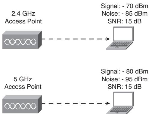
**Figure 11-1** A Case Where the Range Is the Same for a 2.4-GHz and 5-GHz System
