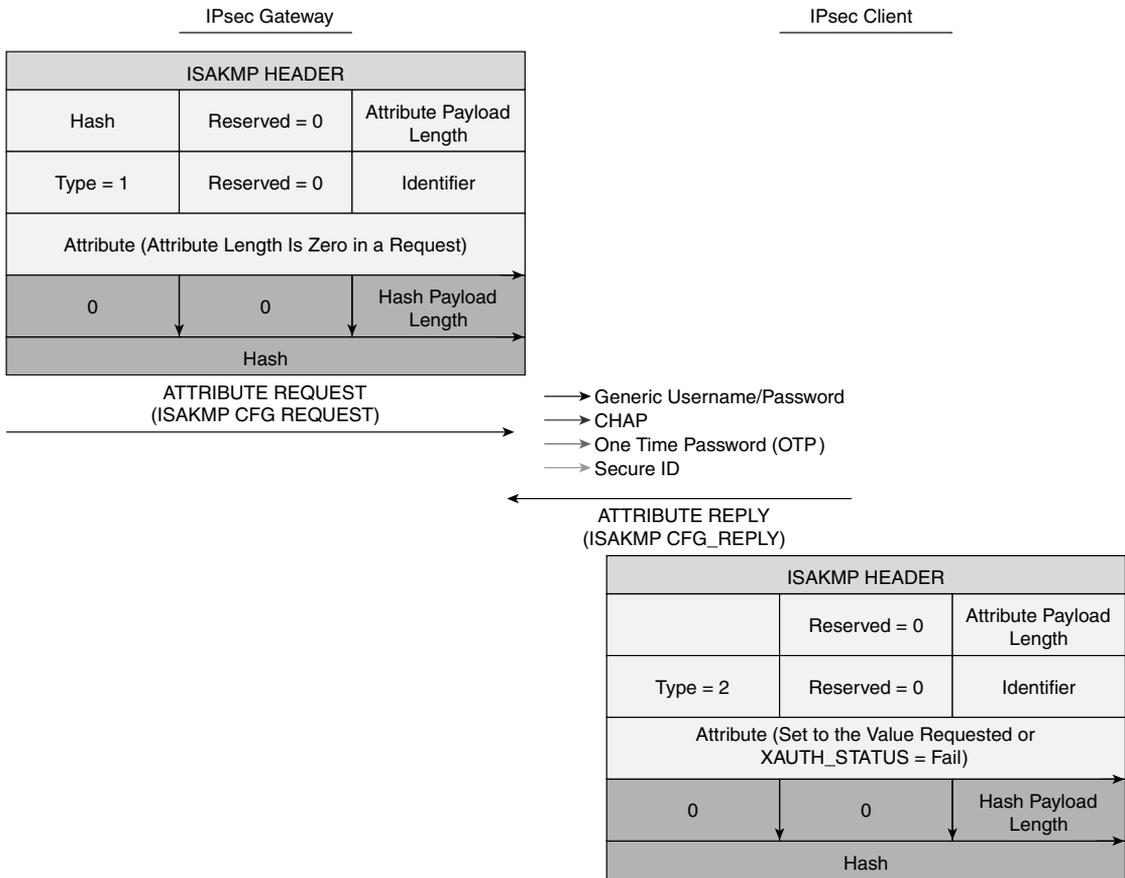
As shown in Figure 4-1, XAUTH uses a Request/Reply mechanism to provide the extended authentication. The XAUTH process is terminated, either when the gateway starts a SET/ACK exchange, which includes an XAUTH\_STATUS attribute, or when the remote device sends a XAUTH\_STATUS attribute in a REPLY message.
