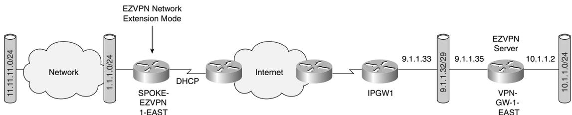
IPsec encapsulates all traffic from the EzVPN client's private network, which is marked as 'inside' to networks behind the IPsec gateway. Therefore, devices behind the gateway have direct access to devices on the EzVPN client's private network via the tunnel and vice versa without the need for NAT or PAT. As there is no reason for NAT or PAT, the EzVPN server does not push down an IP address for tunneled traffic, but all other attributes like ACLs, DNS, and
