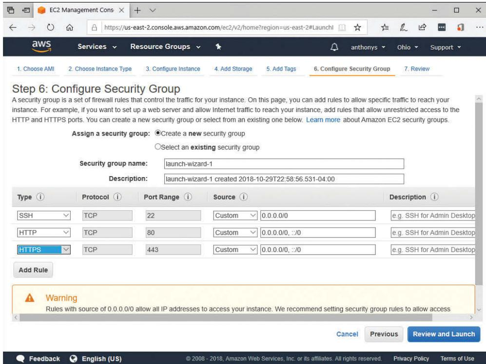
**Figure 12-10** Ensuring Your Security Group Permits the Correct Traffic
