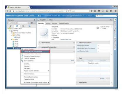
**Figure 12-21** Deploying a VM from a Template
