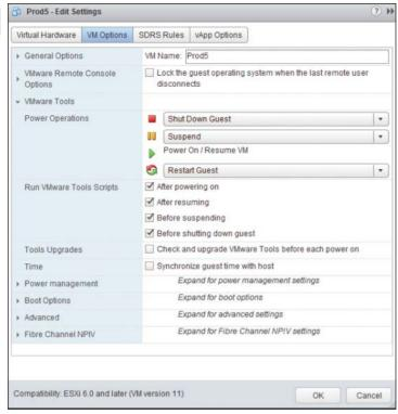
Figure 12-10 VMware Tools Options with VM Powered Off
