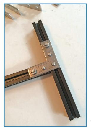
**FIGURE 4.10** Make a "T" with the two beams and secure with a bracket.
