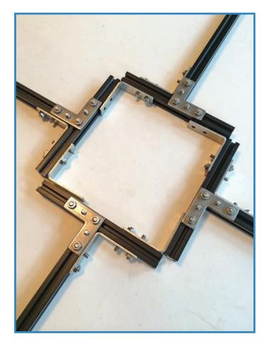
**FIGURE 4.13** Add the four segments together, and you start seeing your airframe take shape.
