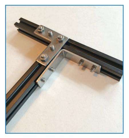
FIGURE 4.11 Reinforce the "T" with another bracket.
