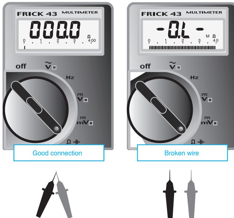
**Figure 4.18** Sample resistance meter readings
