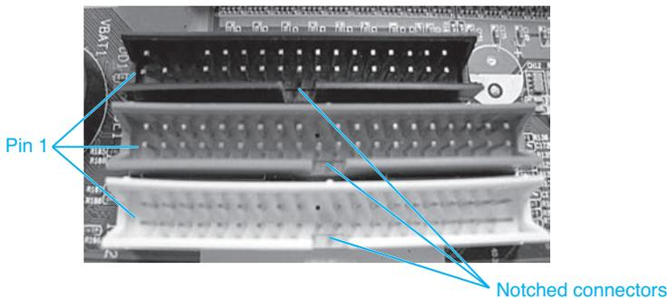
**Figure 4.8** Three motherboard connectors
