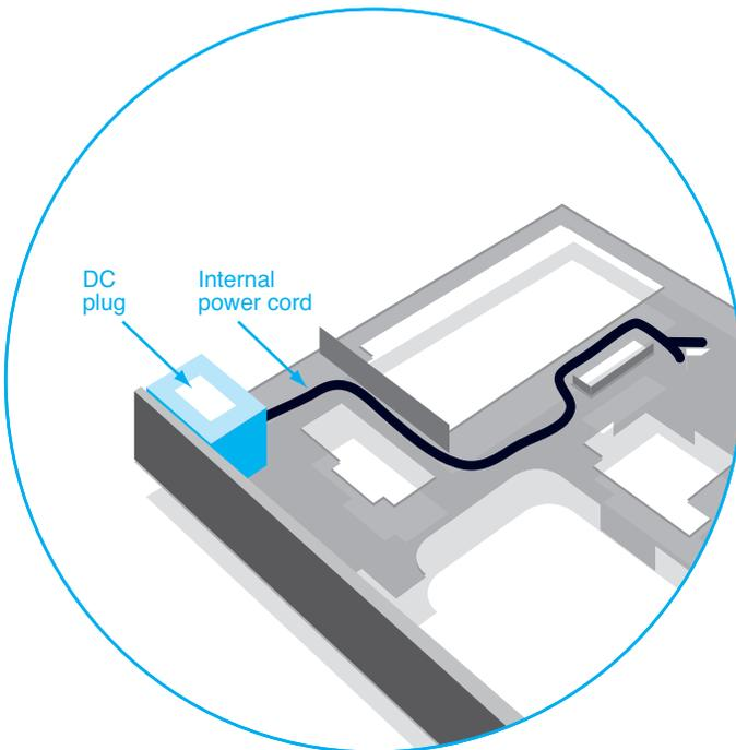
**Figure 4.15** Laptop DC power plug cable
