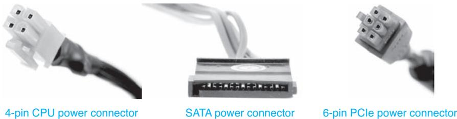
**Figure 4.19** Common power supply connectors
