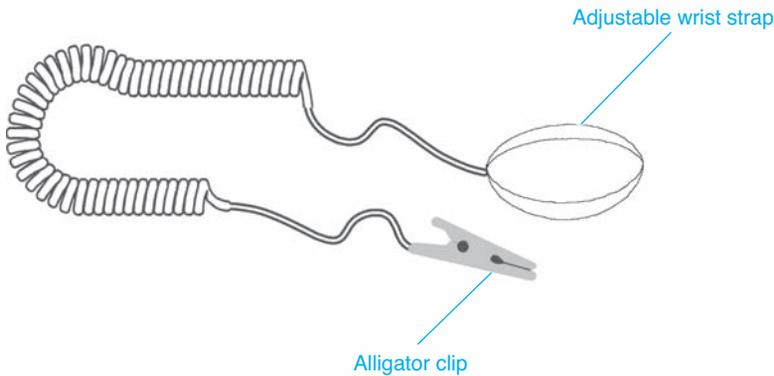
**Figure 4.1** Antistatic wrist strap
