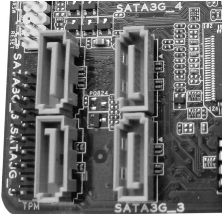
**Figure 4.7** Motherboard connectors for narrow cables
