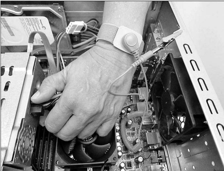
**Figure 4.2** Attaching an antistatic wrist strap
