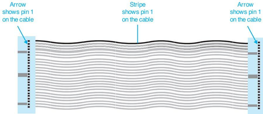
**Figure 4.5** Pin 1 on a ribbon cable
