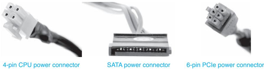
**Figure 4.19** Common power supply connectors
