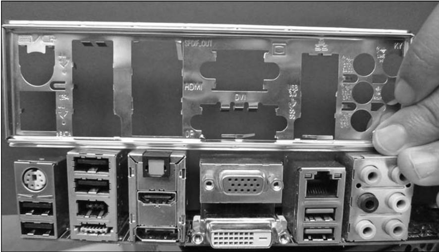
**Figure 4.11** Motherboard I/O shield
