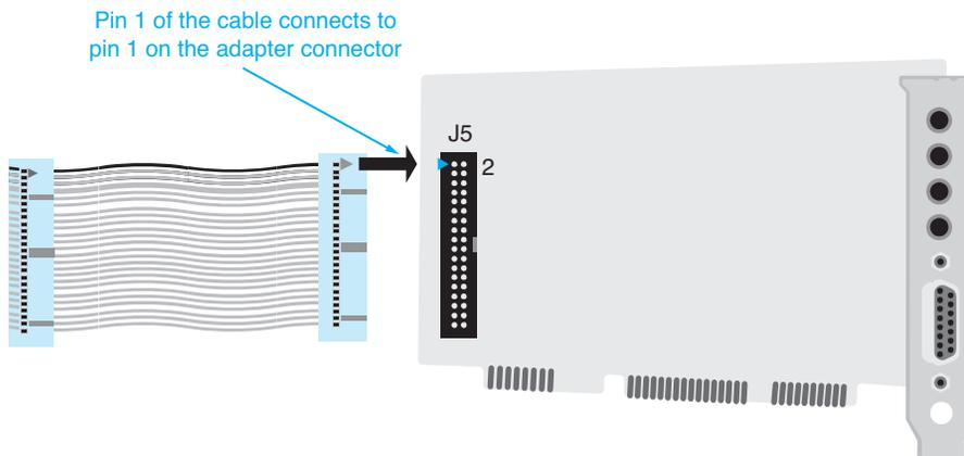
**Figure 4.6** Pin 1 on an adapter
