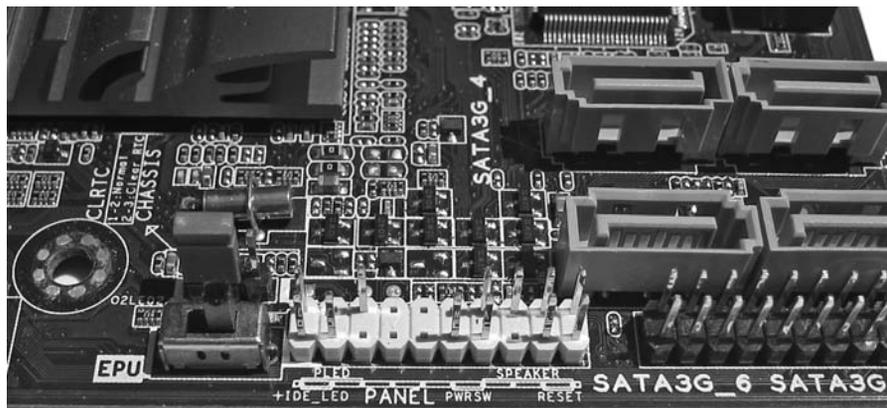
**Figure 4.10** Motherboard front panel connectors
