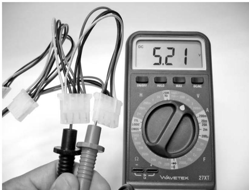
**Figure 4.16** DC voltage reading
