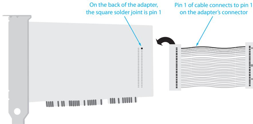
**Figure 4.9** Pin 1 on a connector
