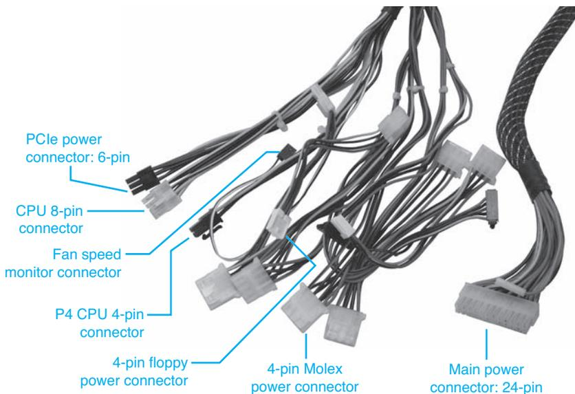
**Figure 4.20** ATX power supply connectors
