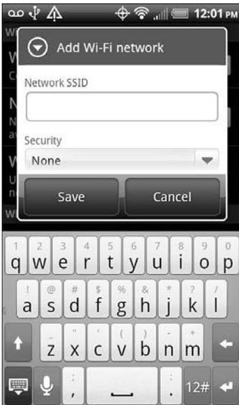
FIGURE 17.4 Android OS Prompting for the user to enter an SSID
