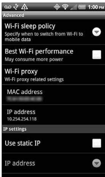
FIGURE 17.7 Advanced wireless settings in Android
