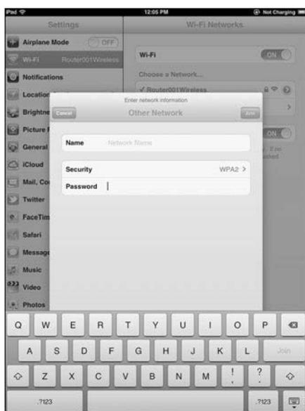
FIGURE 17.5 iOS Prompting for the user to enter an SSID for a WPA2-secured network
