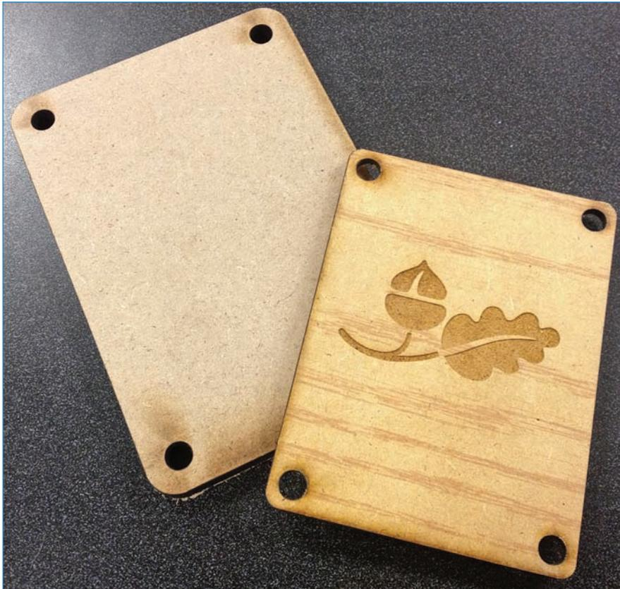
**FIGURE 4.18** I used laser-cut wood for the buzzer unit's enclosure.
