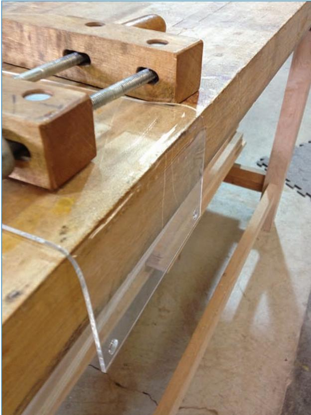
**FIGURE 4.17** As the acrylic heats up, it starts to bend.
