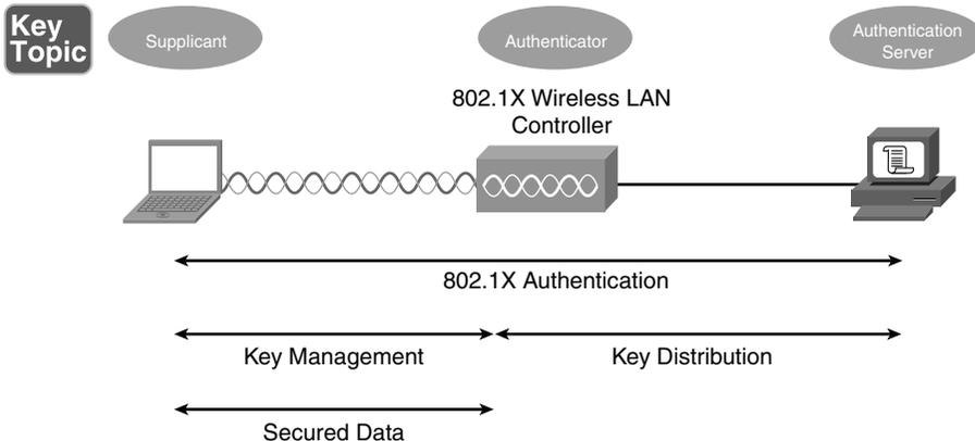
**Figure 8-12** IEEE 802.1x Security for a WLAN
