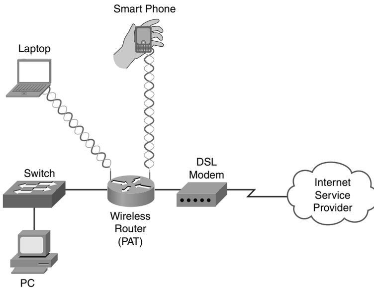
**Figure 8-1** Basic WLAN Topology with a Wireless Router
