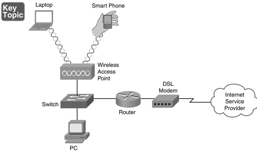
**Figure 8-2** Basic WLAN Topology with a Wireless AP
