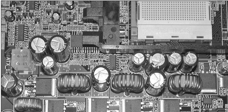
**Figure 3-23** A portion of the VRM on an Athlon 64 motherboard.
