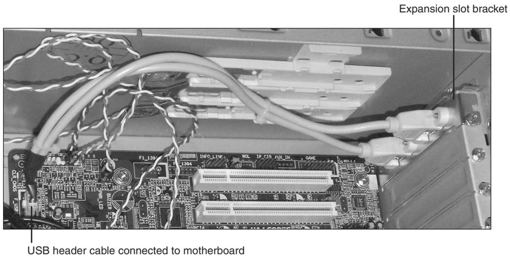
**Figure 3-16** A typical dual-USB header cable that uses an expansion slot bracket.
