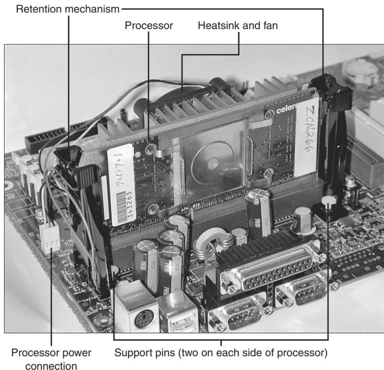
**Figure 3-29** A Slot 1-based Celeron CPU after installation. The heat sink and fan are attached to the rear of the CPU.
