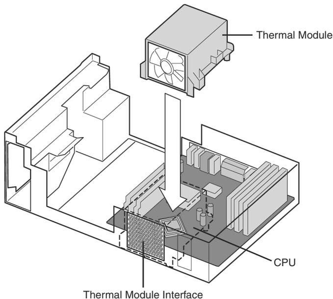
**Figure 3-27** Thermal module placement on a typical BTX motherboard. Figure courtesy of [www.Formfactors.org](http://www.Formfactors.org).
