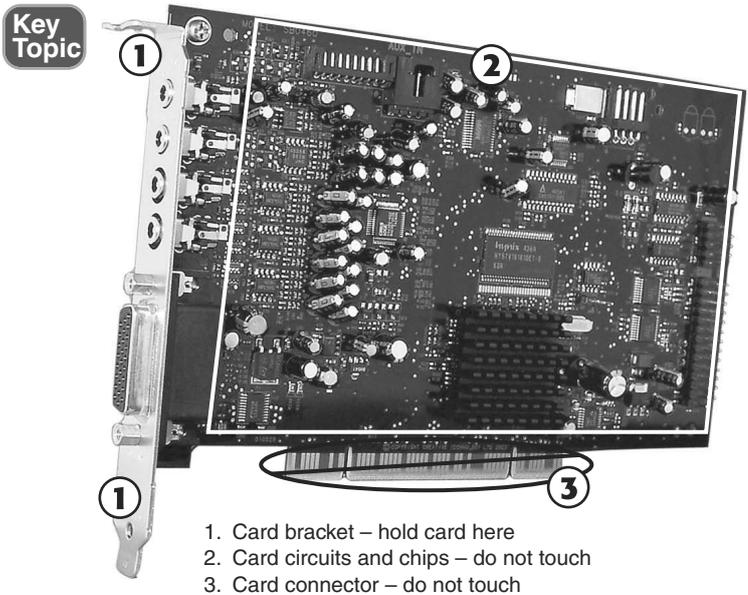
**Figure 3-32** A typical adapter card. Callouts indicate where it is safe and not safe to hold the card.
