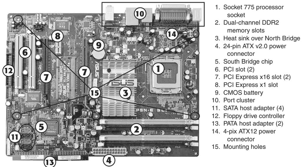
**Figure 3-1** A typical motherboard.
