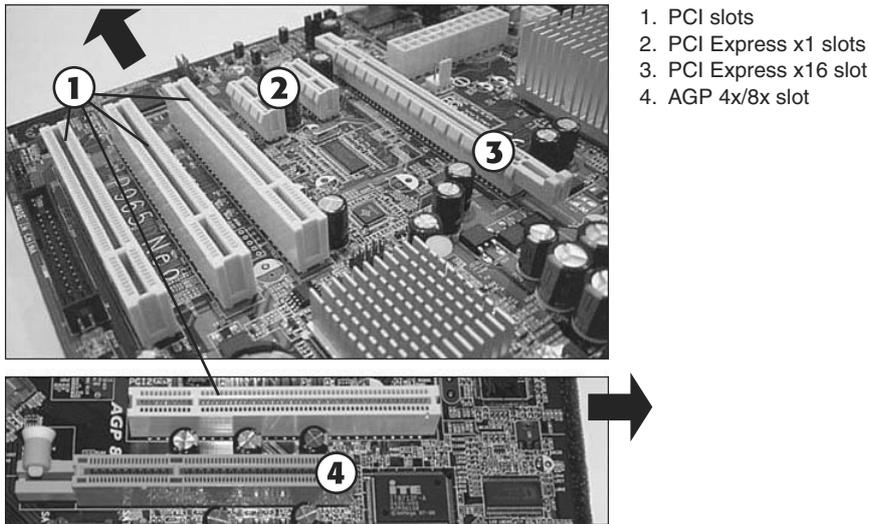
**Figure 3-30** AGP, PCI, PCI Express x1 and x16 slots on typical motherboards. Arrow indicates rear of motherboard.
