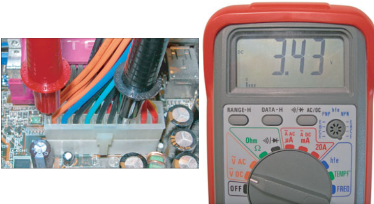
FIGURE 5.11 Testing the 3.3\text{V} wire with a multimeter set to volts DC
