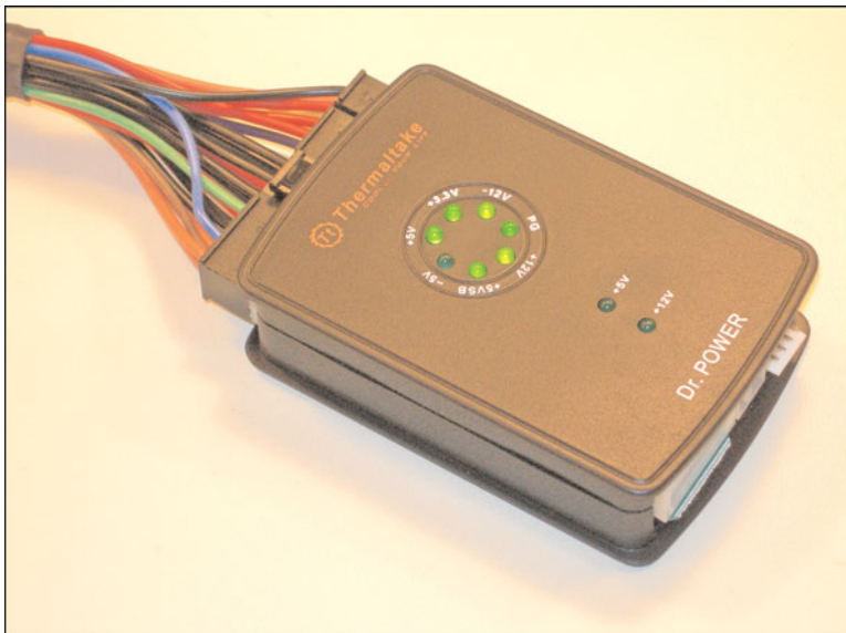
FIGURE 5.10 Testing a 24-pin P1 connector with a power supply tester
