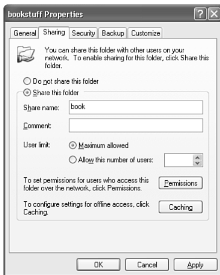
Figure 6.12 When Simple File Sharing is not active, there are more specific permission controls.
