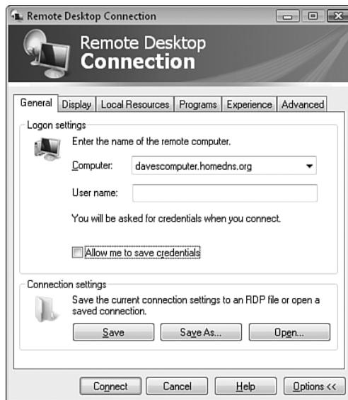
**Figure C.9** The Remote Desktop Connection dialog lets you configure the connection and select the remote computer to use.
