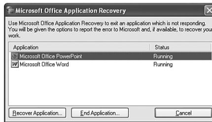
Figure 3.10 If an Office program quits responding, try to use the Application Recovery utility to recover your work.
