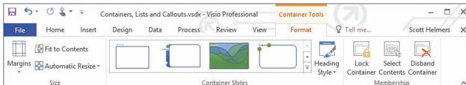
Figure 13-7 The Format tool tab appears only when you select a container
