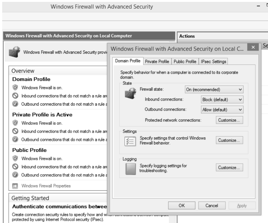
FIGURE 3-15 Use the Windows Firewall With Advanced Security dialog box to configure settings for specific profiles.
