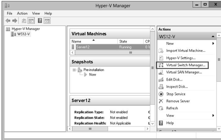
**FIGURE 3-15** Opening the new Virtual Switch Manager
