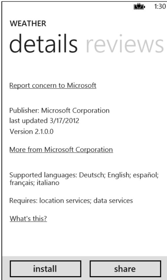
**FIGURE 1-5** Security capabilities are displayed as user-readable strings in an app's details page.
