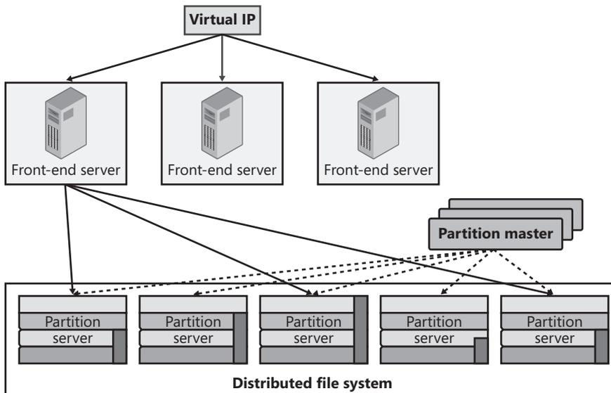
**FIGURE 2-3** Windows Azure storage architecture consists of a front-end Virtual IP and three basic layers.
