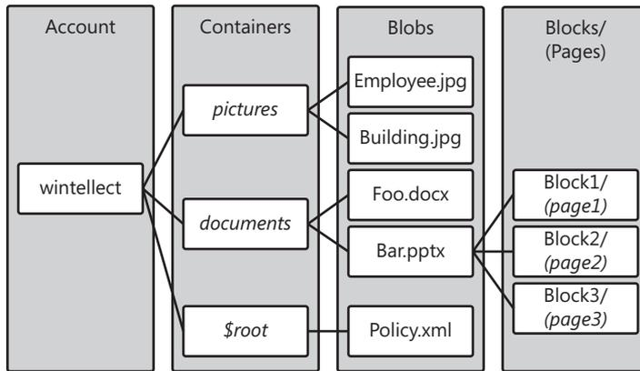
**FIGURE 5-2** The blob storage structure is a hierarchical relationship between storage accounts, blob containers, blobs, and pages.
