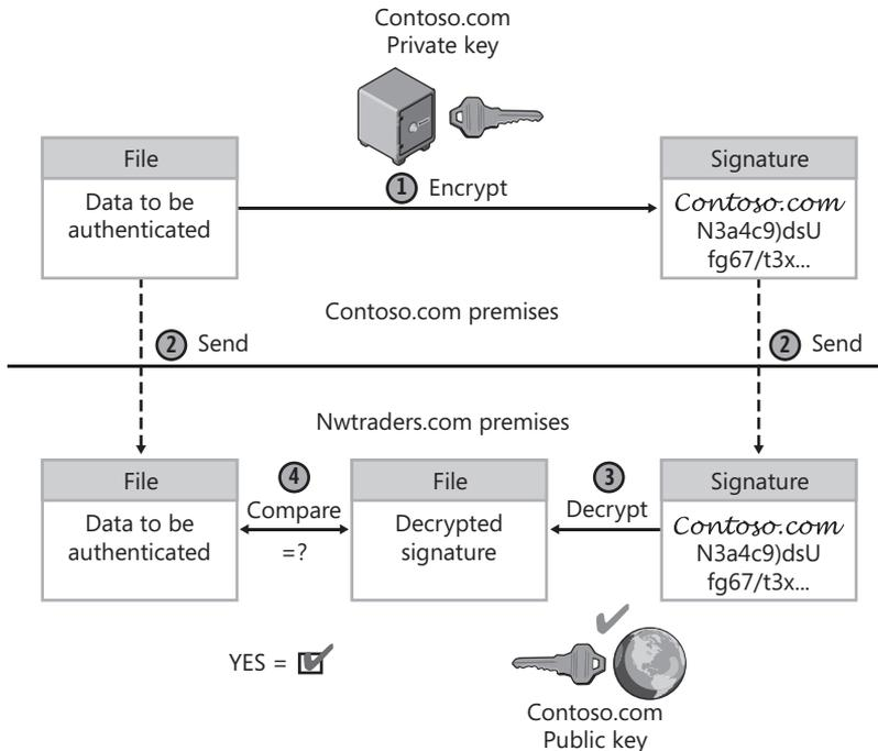
**FIGURE 3-36** Creation and verification of a digital signature
