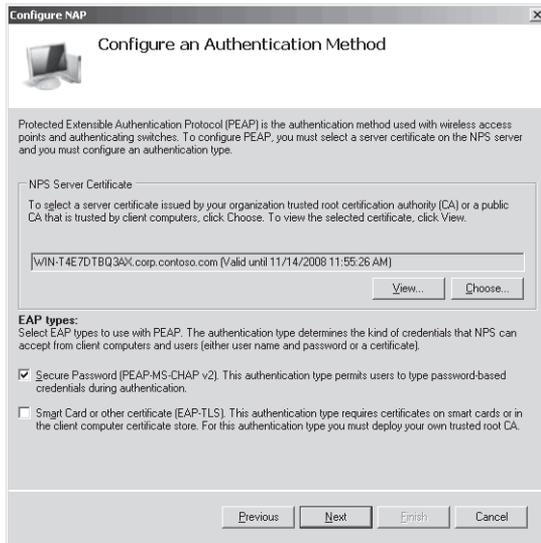
**FIGURE 8-4** Configuring an 802.1X enforcement authentication method
