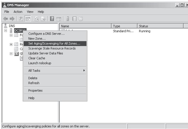
**FIGURE 3-16** Enabling aging at the server level
