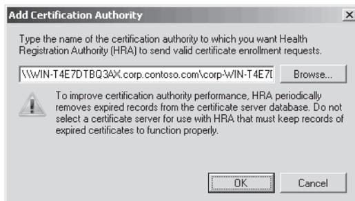
**FIGURE 8-6** Selecting a CA for IPsec enforcement
