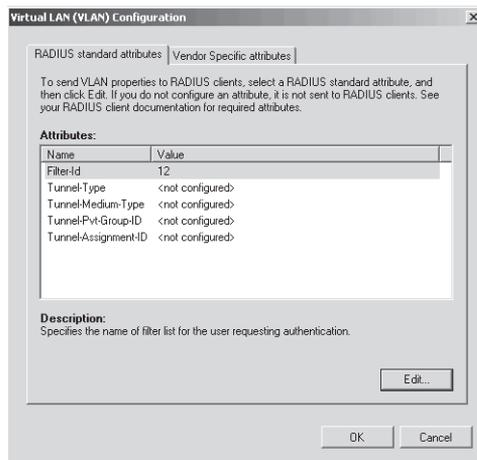
**FIGURE 8-8** Configuring the VLAN for unrestricted network access
