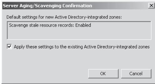
**FIGURE 3-17** Enabling aging on Active Directory-integrated zones
