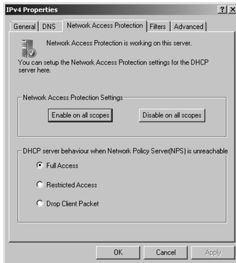
**FIGURE 8-9** Configuring NAP on a DHCP server
