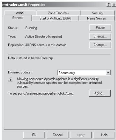
**FIGURE 3-18** Accessing aging properties for a zone
