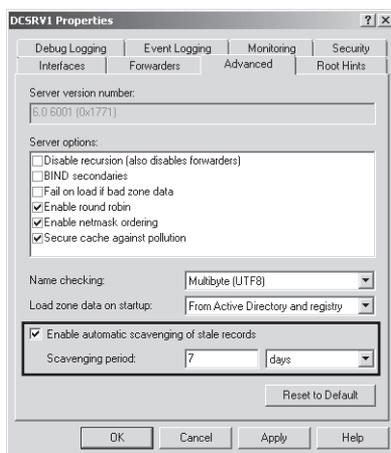
FIGURE 3-20 Enabling automatic scavenging on a DNS server
