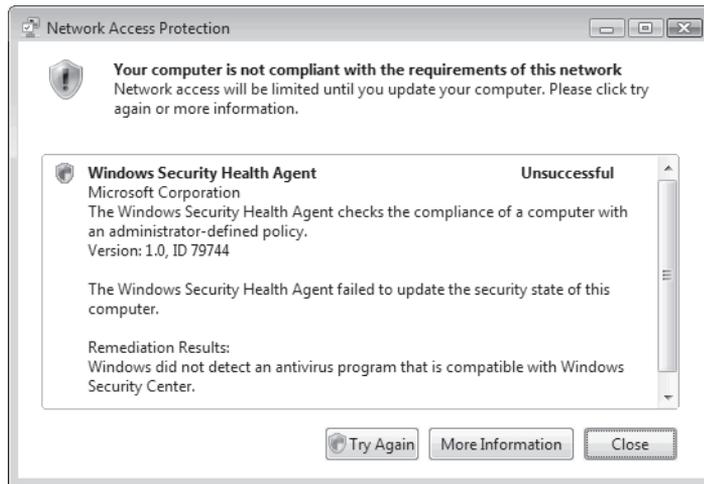
**FIGURE 8-14** Information provided to a noncompliant NAP client
