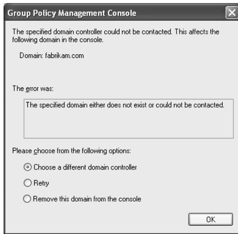
Figure 4-2 When the domain controller running the PDC emulator role is not available for editing the GPO, an error message appears.
