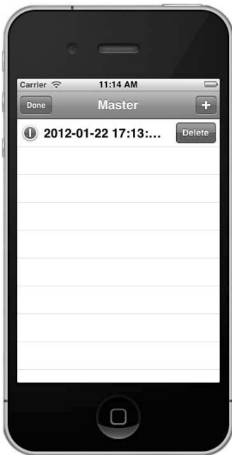
FIGURE 8.4 The skeletal code that comes with the Core Data + Master-Detail Application project template is enough to produce an app that can run in the iOS Simulator. It can add rows to its table, and, as shown here, respond to the Edit button by offering to delete rows.
