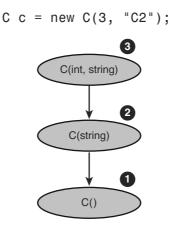
FIGURE 3.7 Constructor chaining sequence
