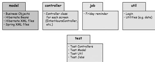
Figure 3.6 UML package diagram for Time Expression.
