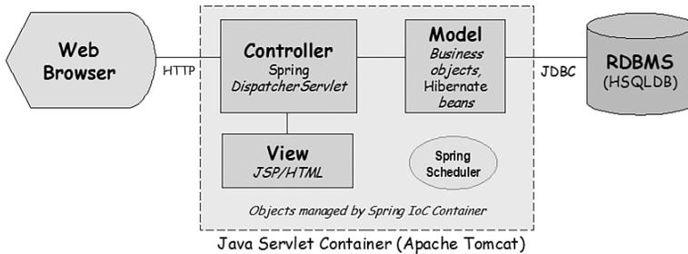
Figure 3.2 High-level architecture for Time Expression.
