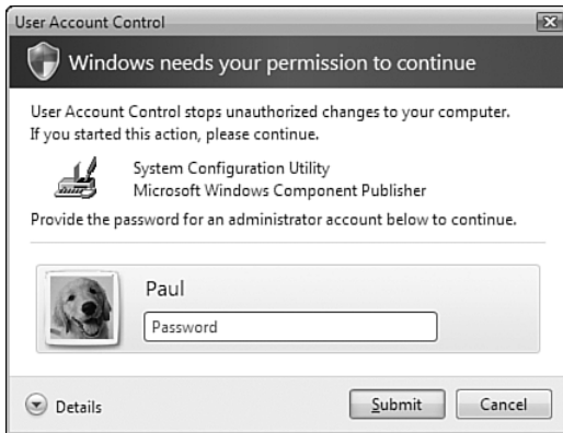
FIGURE 6.2 When a standard user launches a task that requires administrative privileges, Windows Vista displays this dialog box to ask for administrative credentials.
