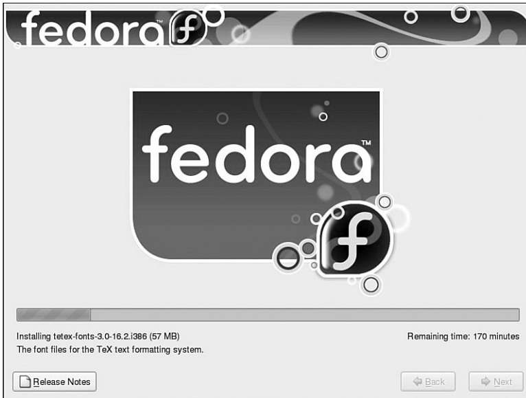
FIGURE 3.18 The Fedora installer formats your drive, and then installs selected software package groups.
