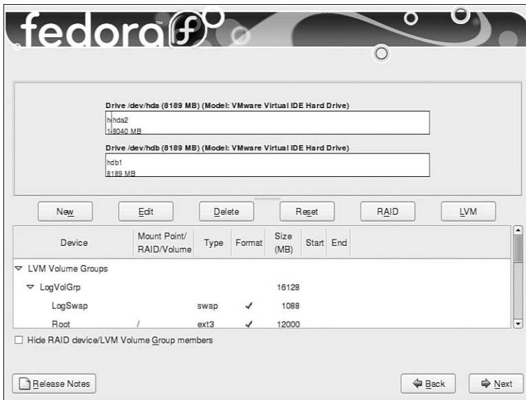
FIGURE 3.11 The completed masterpiece. It is worthwhile spending extra time to get the best partition layout for your requirements.
