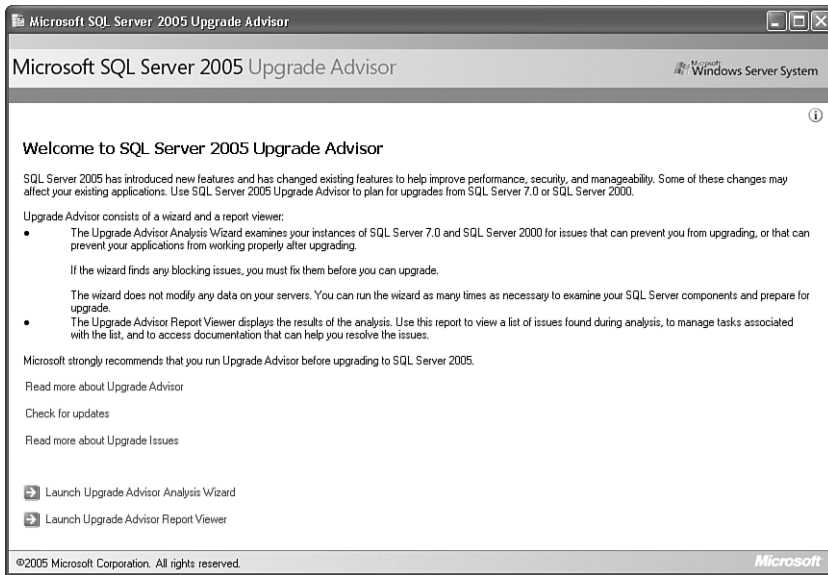
FIGURE 3.2 The Upgrade Advisor lets you view reports or run the Upgrade Advisor Analysis Wizard.
