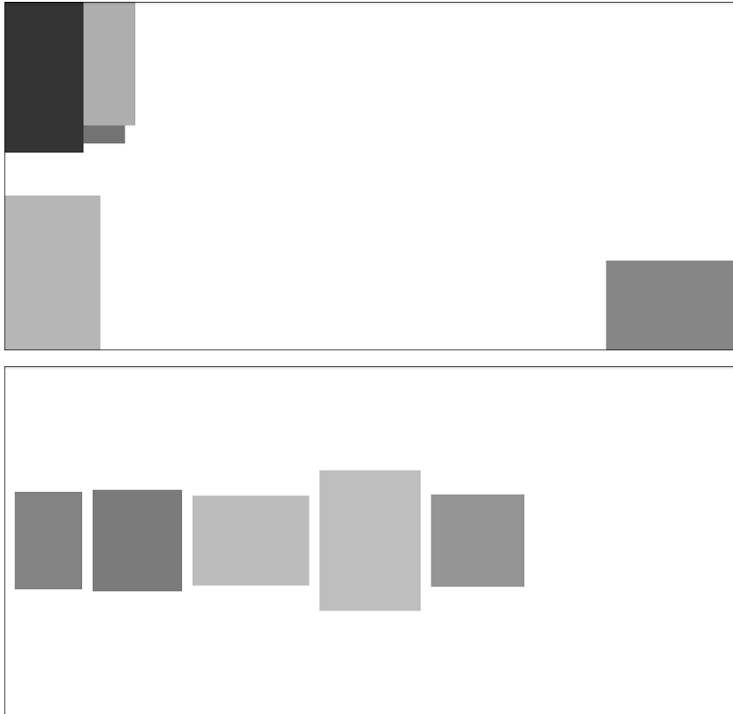
Figure 1-3 Odd layout positions (top) are the hallmark of an underconstrained layout. Although these particular views are constrained to show up onscreen, their near-random layout indicates insufficient rules describing their positions. By default, views might not show up at all, especially when they are underconstrained. Chapter 4, “Visual Formats,” discusses fallback rules, which ensure that views are both visibly sized and onscreen. A sufficient layout (bottom) provides layout rules for each of its views.
