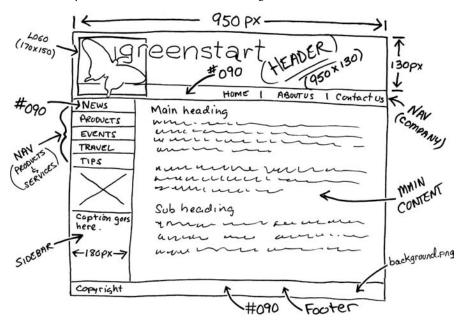
The wireframe for the final design should identify the components and feature markup for content, color, and dimensions. ► Tip: For years, designers have started the design process in Fireworks, where they can create a fully functional mockup that can then be exported to a CSS-based HTML layout and then edited in Dreamweaver.
