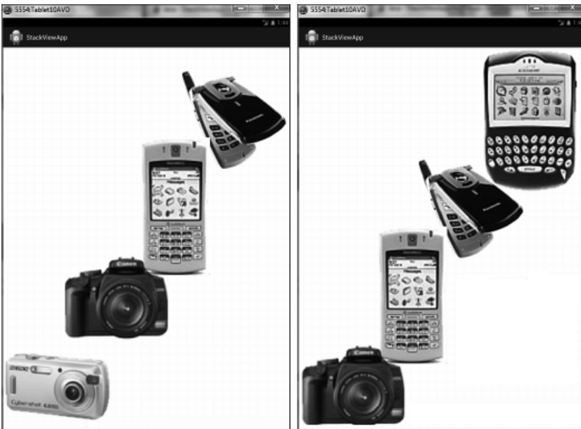
Figure 4.5 stackView displaying enlarged images (left); the images at the back appear in the front when you flip the front images (right).
