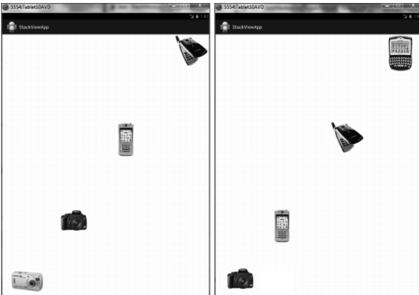
Figure 4.4 StackView displaying images (left), and the hidden images displayed in the front after flipping the front images (right)
