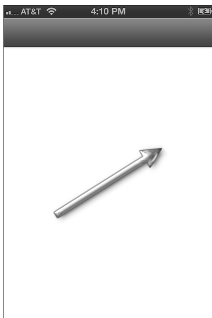
Figure 1-1 A little math recovers the “up” direction by performing an arctan function using the x and y force vectors. In this example, the arrow always points up, no matter how the user reorients the iPhone.
