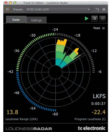
**Figure 4.32** The Loudness Radar effect is new in Adobe Premiere Pro CC. It lets you ensure that your program is compliant with broadcast standards.
