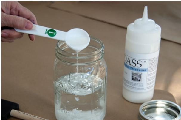
**FIGURE 4.3** Add the concentrate to the alcohol—not the reverse!
