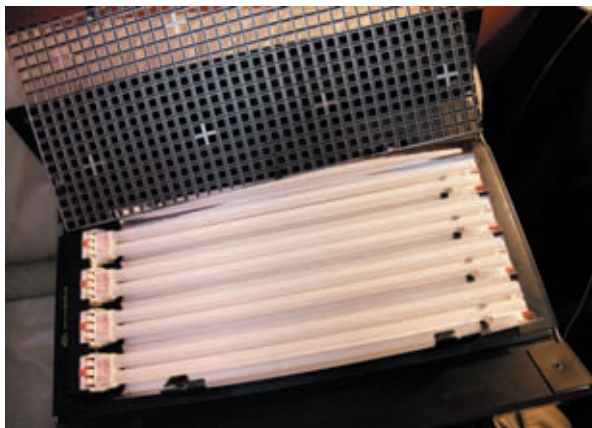
▲ Fluorescents like this Kino Flo Diva make a soft, pleasing key light.
