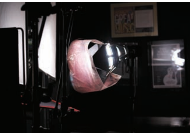
▲ A correction gel (1/2 CTO) is added to a day-light-balanced HMI to warm up its output.
