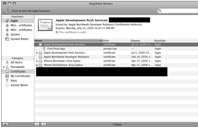
Figure 16-5 Identify which Push Service SSL certificate you are dealing with by clicking the down arrow. This reveals the common name used to generate the original certificate request.
