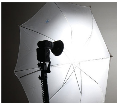
⌘ Figure 3: The flash is too close to the umbrella
