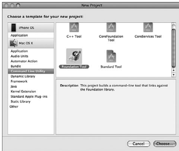
Figure 2.4 Starting a new project: creating a Foundation tool
