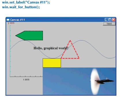
Note how the parts of the photo that didn't fit in the window are simply not represented. What would have appeared outside the window is "clipped" away.
