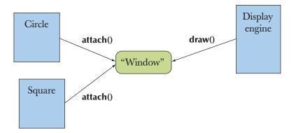
The "display engine" draws lines on the screen, places strings of text on the screen, colors areas of the screen, etc. For simplicity, we'll use the phrase "our GUI library" or even "the system" for the display engine even though our GUI library does much more than just drawing the objects. In the same way that our code lets the GUI library do most of the work for us, the GUI library delegates much of its work to the operating system.
