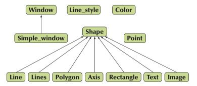
An arrow indicates that the class pointing can be used where the class pointed to is required. For example, a **Polygon** can be used where a **Shape** is required; that is, a **Polygon** is a kind of **Shape**.
