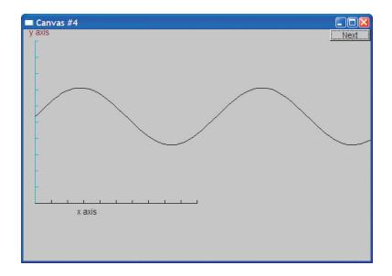
Note how the curve simply stops when it hits the edge of the window. Points drawn outside our window rectangle are simply ignored by the GUI system and never seen.
