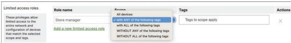
**Figure 4-30** Entering Name and Scope to Create a Limited Access Role
